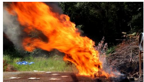
Western juniper tree burning as part of an effort to identify properties that control ember generation.
