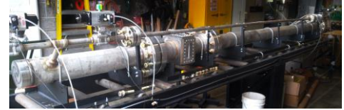
Detonation tube with optical access.
