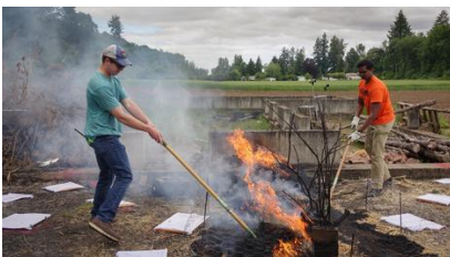
Figure 2. Burning of chamise to study firebrand production.
