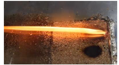
Figure 4. Smoldering to flaming transition in a wind
