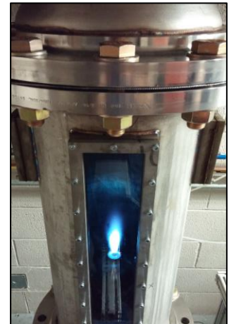
Turbulent Bunsen burner burning jet-like fuel at 0.6 atm.
