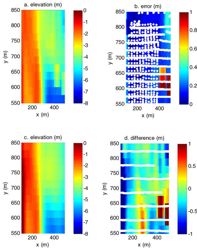
Fig. 14. Comparison of bathymetry derived using (a) 2-D wavenumber estimates and (c) surveyed (and spatially interpolated) bathymetry. Maps show (b) the predicted errors from the wavenumber inversion and (d) the actual differences between wavenumber inversion and survey. White dots on the error maps indicate the sample locations for both (b) imagery and (d) survey data sets.
