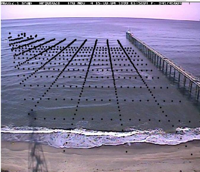
Fig. 4. Camera view of the Duck field site, showing the image time series sample locations (black dots). The camera orientation and distortion are used to map the data to georeferenced locations. The cameras are mounted on a tower, whose shadow on the beach provides a self-portrait.
