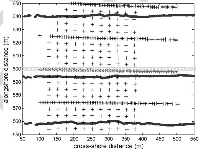
Fig. 5. Duck sampling pattern with the shoreline at the left near  $x = 100$ . Bathymetric survey locations are indicated by dots (very densely spaced in the cross-shore direction); image time series (+) were sampled over the 2-D domain. The samples used in the 1-D analysis are indicated with bold symbols. Wavenumbers were estimated on a sparse tomography domain, which is indicated by circles (1-D case).
