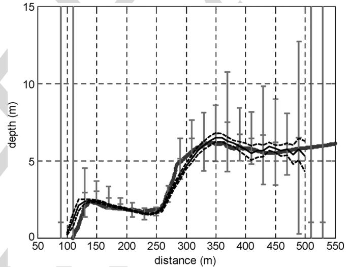
Fig. 13. Water depth estimated from image-derived wavenumbers. The estimates from the 1-D wavenumber inversion are shown with error bars and the estimates from the 2-D analysis are shown as a solid line with dashed lines, indicating one standard deviation error. The nearest survey observations are shown as blue dots.
