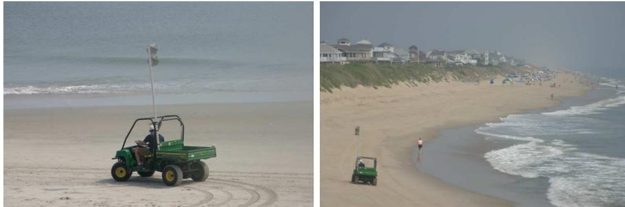
**Fig. A.1:** ATV with the corner reflectors mounted. The optical contrast of the ATV with the beach is readily noticeable.
