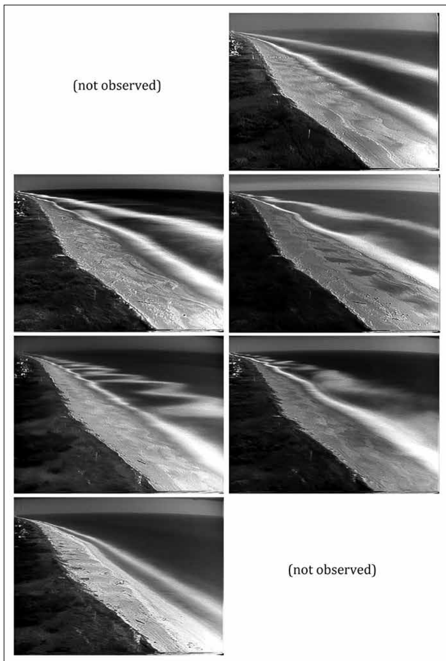
Figure 7. Optical time-exposure images from Duck, NC, showing the range of morphologies observed over time at one site. These morphological classes could be loosely related to wave forcing (from Lippmann and Holman [1990]).
