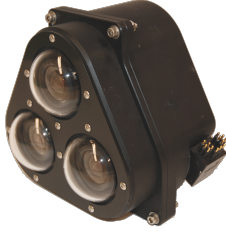
Fig. 3: The Trisect underwater perception system developed by UW-APL includes two 5MP monochrome machine vision cameras for stereopsis, with a 12MP color camera for color overlay. Point clouds are calculated onboard the sensor by an NVidia Xavier NX processor and published via ROS.
