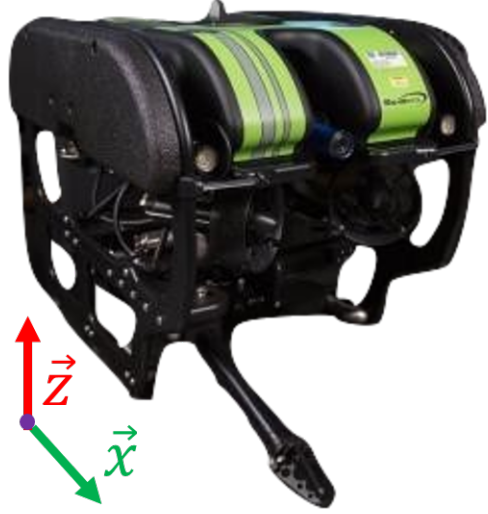
Fig. 2. A SeaBotix vLBV300 ROV similar to the one modeled in this work. Along with IMU and DVL sensors, the vehicle has six angled thrusters which control it along five degrees of freedom: heave (vertical z ), sway (lateral y ), surge (lateral x ), roll (rotation around x ), and yaw (rotation around z ). For this work, only the x and z axes are considered.
