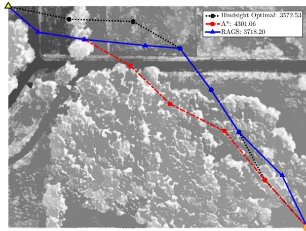
**Fig. 6.** Paths are planned through a dense cluster of trees surrounding the goal. Here we can see RAGS plans around the cluster, where there are more low cost paths, before traversing through a less cluttered area. RAGS takes advantage of the wide open region instead of searching for narrow tracks within the tree cluster.
