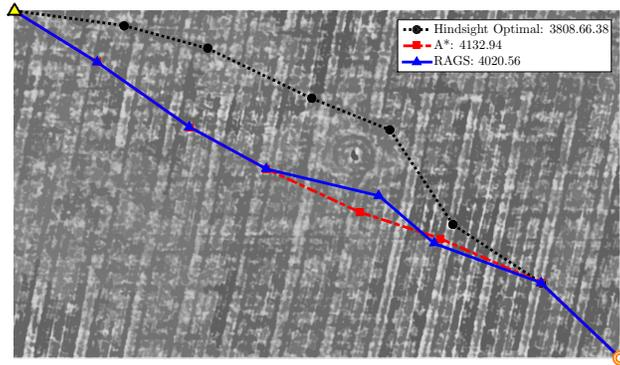
**Fig. 5.** The RAGS,  $A^*$ , and the global optimal (known only in hindsight) paths are shown in the figure with the final path costs. The goal is to traverse from the top left start vertex to the bottom right goal vertex. The empty field is a test case showing that both algorithms plan direct paths as expected in an obstacle-free environment.
