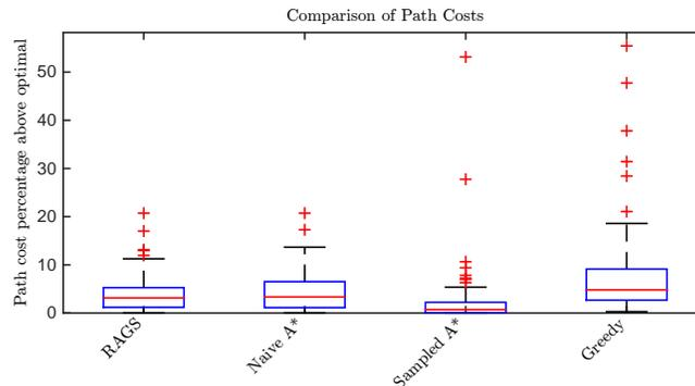
**Fig. 8.** Results from satellite data experiment, using 100 images. Box plots represent the path cost percent above what would have been in hindsight the optimal path. The same trends in performance are seen as with the simulated graphs. RAGS accounts for uncertainty in traversing the world, balancing risk of travel time (cost) to reduce expensive outliers seen in the comparative algorithms.
