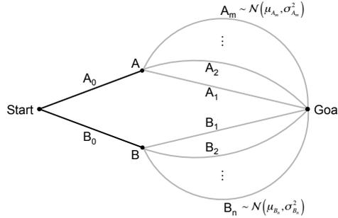
**Fig. 1.** Setup of pairwise comparison for sequential lookahead planning. Given the path cost distributions, we can directly compute the probability that traveling from Start to Goal through A will ultimately yield a cheaper path than traveling via B.
