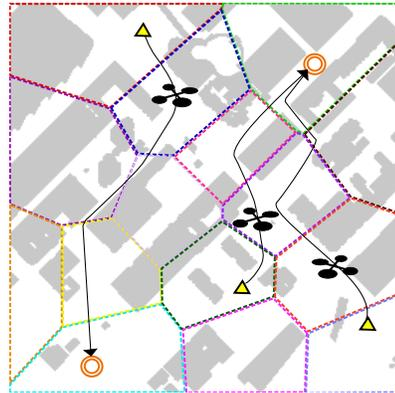
Fig. 1: The UAV traffic management problem. The airspace is divided into discrete sectors with a single UAV traffic management (UTM) agent controlling the cost of travel through each sector. UAVs traveling from start (triangle) to goal (circle) locations plan and execute paths to reduce their individual travel cost without explicitly coordinating with other UAVs in the airspace.
