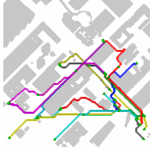
Fig. 4: Initial planned paths for 27 UAVs in the airspace travelling from start (solid green triangle) to goal (solid green circle) locations. It can be seen that high levels of congestion may be expected in some thoroughfare regions of the airspace, such as the bottom right area where there are a group of close fixes.
