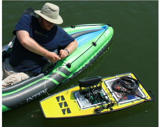
Fig. 1: Commanding aquatic robots, such as the pictured Platypus Lutra autonomous surface vehicle, is currently a slow, hands-on process where operators manually set individual waypoints at the outset of the mission. This burden motivates the need for algorithms that can quickly learn and meet a human operator’s goals while adapting to the dynamic aquatic environment.
