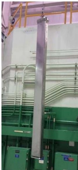
Crane-Suspended Handling Mockup in Front of Reactor
