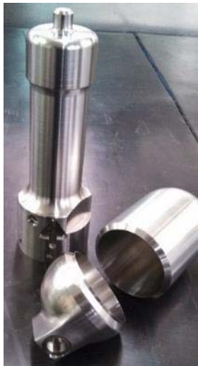
1 of 4 fabricated prototype vessels (welding to be performed)
