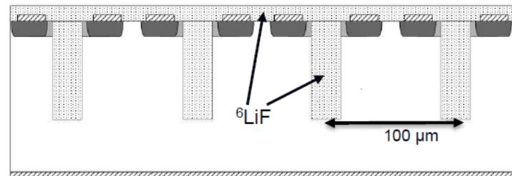
100 micron pixel pitch (center to center), each 1-D pixel read out separately
