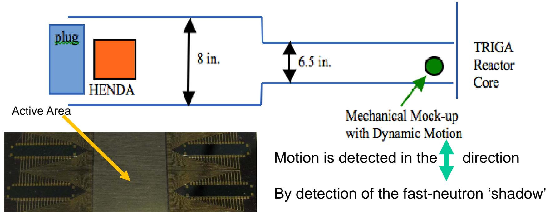
Active area has no electronics behind it -- flexible connectors allow electronics to be shielded from neutrons
