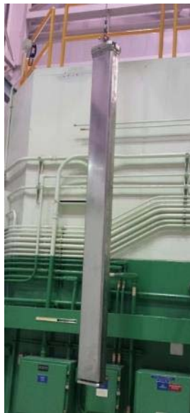
Crane-Suspended Handling Mockup in Front of Reactor
