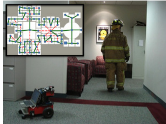
Figure 1: Pioneer robot searching a building with a team of volunteer firefighters. A graphical representation of the building is shown in the top left. The robot and humans coordinate using a provably near-optimal distributed algorithm that combines submodular optimization and pursuit-evasion [9, 10, 15, 20].
