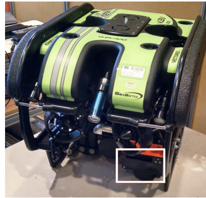
Fig. 4: The Seabotix vLBV300 and Gemini 720i imaging sonar (white rectangle in the lower right) used in experiments.
