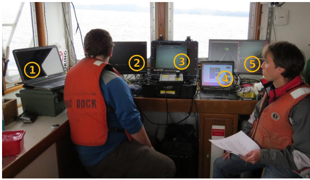
Fig. 2. sAUV control station, including sonar visualizer (far left, 1), Greensea navigation console (2), manual control console (3), ROS data interface (4) and ROS rviz visualization (5).
