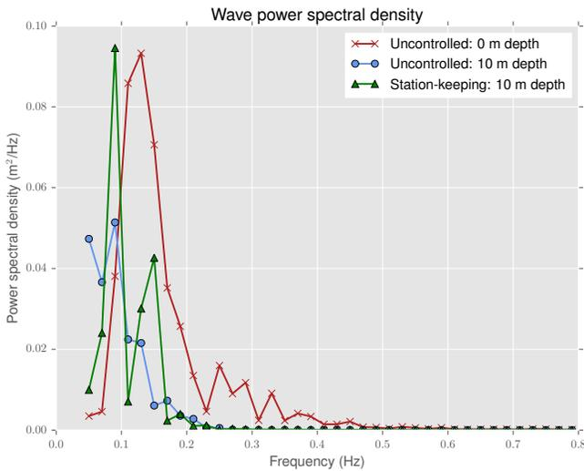
Fig. 5. Wave power spectra generated by recording vehicle vertical displacement when uncontrolled at the surface and 10m depths.
