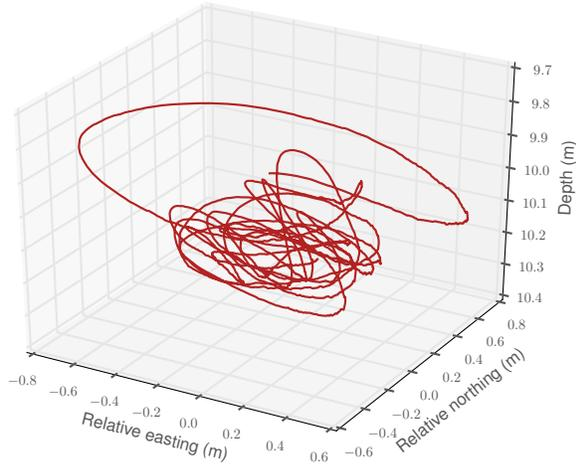
Fig. 7. Station keeping vehicle displacement at 10m depth.
