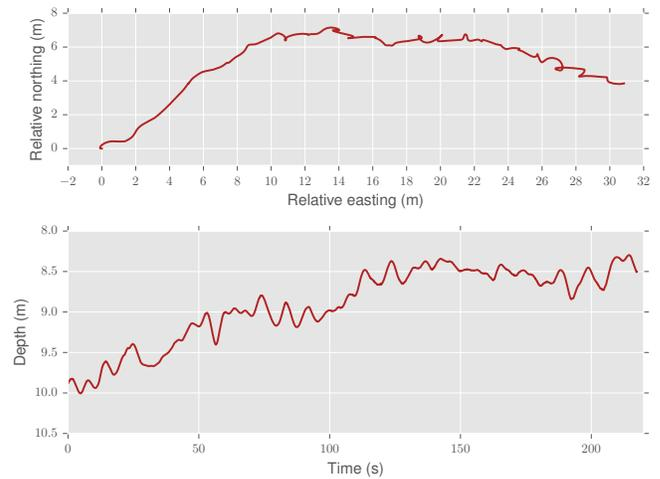
Fig. 6. Uncontrolled vehicle displacement at 10m depth.
