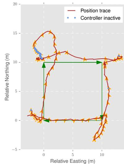
Fig. 12. Vehicle moving around a commanded 10 m square pattern at 40 m depth.
