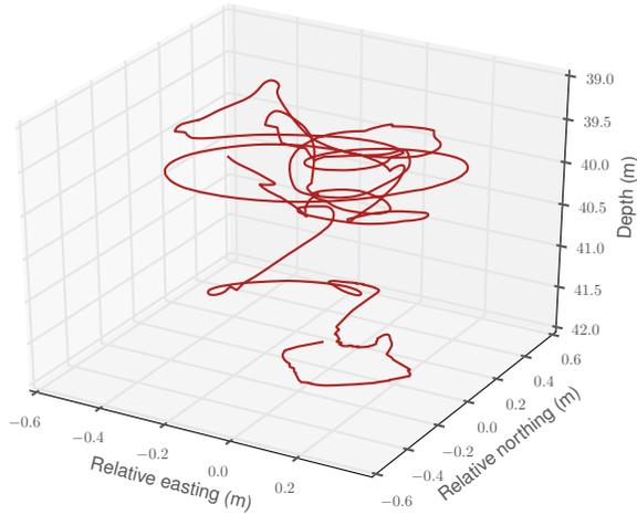
Fig. 8. Station keeping vehicle displacement at 40m depth.
