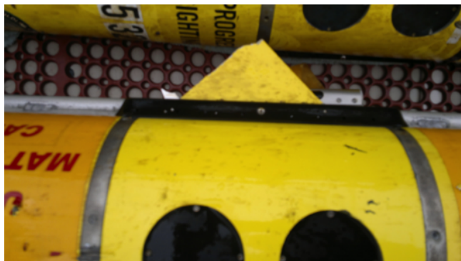
Fig. 1: An autonomous underwater glider [18] that was damaged by ship traffic. These kinds of accidents motivate the need for a better risk-aware path planners informed by human scientists.
