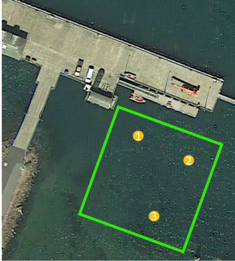
Figure 6.2: An example scenario of the Seabotix vehicle test domain at Newport, Oregon. The yellow circles represent the waypoints and the green box represents the “no go zones”.
