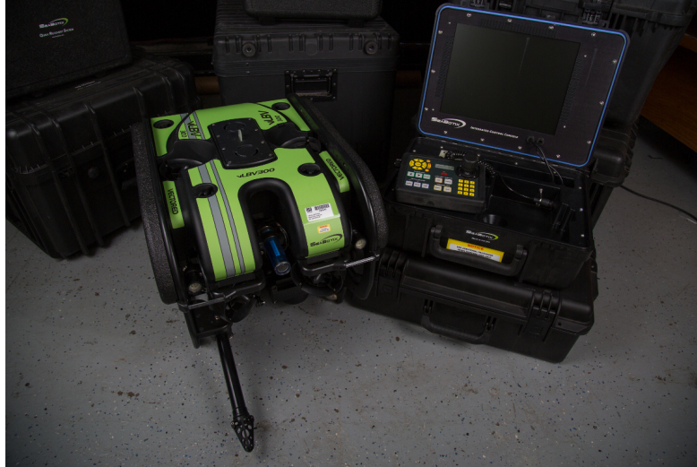
Figure 6.1: The Seabotix vLBV300 used in the field demonstration.
