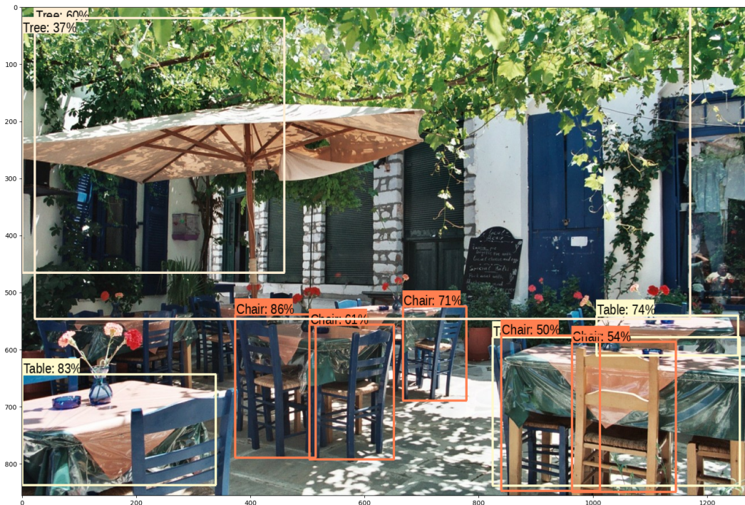
Figure 2.1: Example image containing labeled bounding boxes for detected trees, tables, and chairs from the TensorFlow Object Detection Tutorial. [1]
